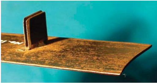
Airfoil #12 - the Wright Brother's original airfoil model from The Franklin Institute.
