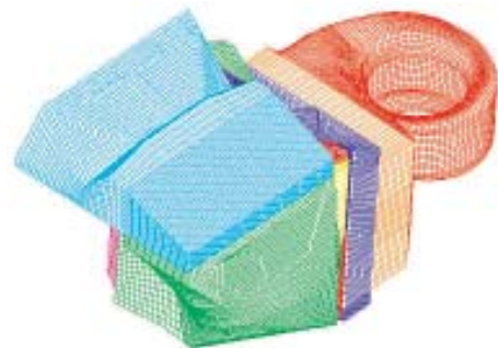
Pointwise uses Gridgen to rapidly generate hexahedral grids for Behr.
